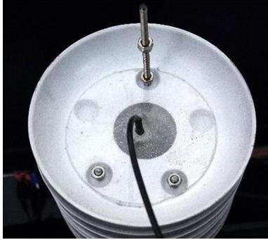
Now spray paint all seven carpet shields white prior to assembly. Spray paint the plastic 90° conduit at the same time.
