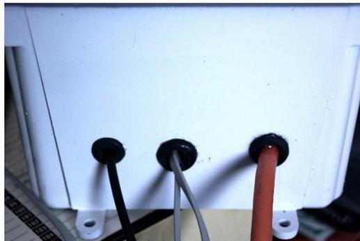
The temperature sensor hole is  $\frac{1}{4}$ " and the other two holes are  $\frac{1}{2}$ ".
