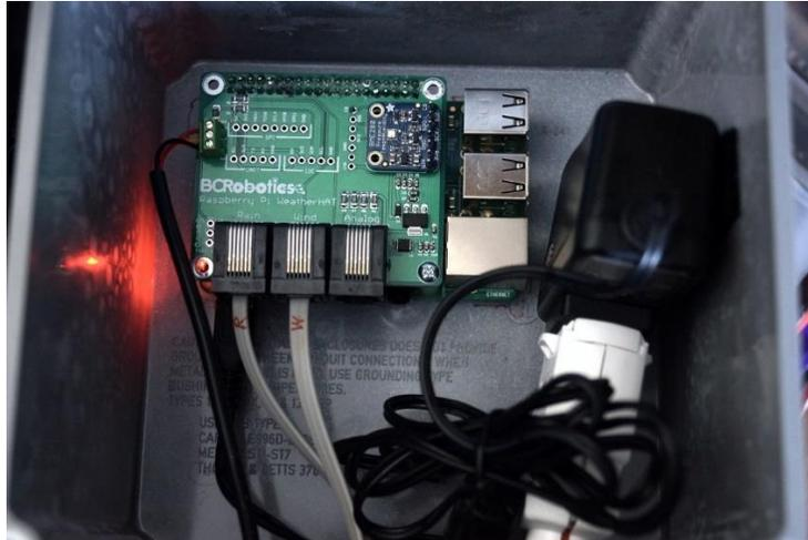
Place it in the top left portion of the box so that there is room for making connections, and room for the power cube. This also helps to keep it dry. The power cube is Velcroed to the side of the junction box so that it does not move inside the box.
